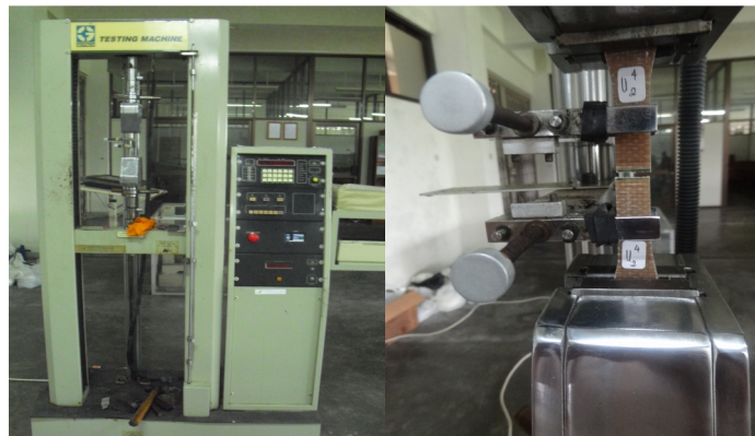
Gambar 2. Go Tech Universal Testing Machine
